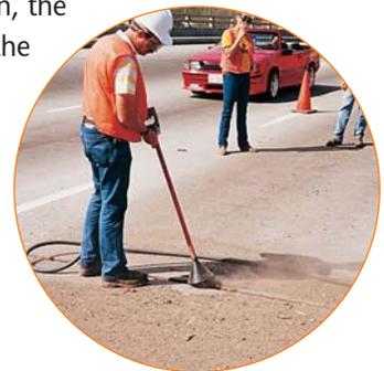
The Soil Pick requires no periodic maintenance. A pressure gauge on the handle assembly advises the operator if the tool is working at acceptable pressure. The Soil Pick weighs 6.5 lbs., has zero hand/arm vibration and can be used for extended periods without fatigue.
