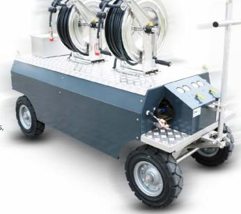
14594. The ARGO is fitted with an integral stainless steel control panel as standard, that comes with two 0-10 bar reducer valves and a high- and low-pressure manometer, as well as a mechanical residual pressure signal by means of a whistle.
