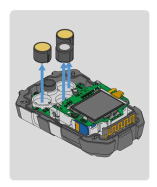
3. Remove the sensor(s) you plan on replacing by pulling it up and clear of the bracket.
