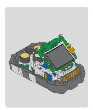
3. Remove the display PCBA and display assembly by lifting it up.
