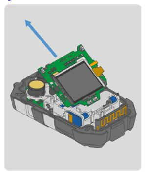
4. Lift the display PCBA and display assembly away from the main board at the angle shown.
