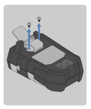
2. Remove the two screws with a Phillips head #1
