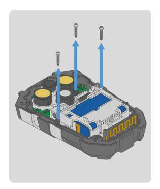
5. Remove the three internal screws with a Torx T6 screwdriver.
