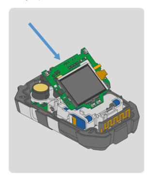
5. Take the new display PCBA and display assembly, and insert the bottom left edge under the snap fit on the battery holder. Push the display PCBA down to engage the board to board connector.
