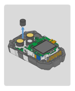
5. Remove the horn by pulling it up and out of the clear bracket.
