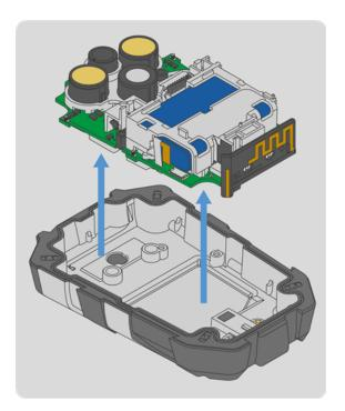
6. Lift the clear bracket and mainboard out of the back housing. Discard the back housing according to local regulations.
