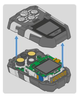
2. Remove the front housing and attached sensor gasket.
