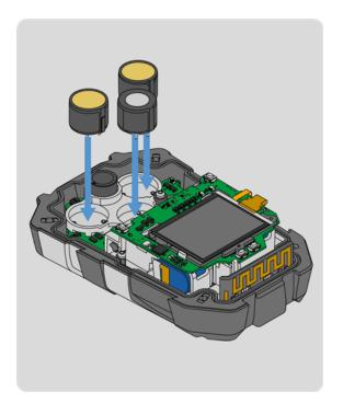
4. Install the replacement sensor(s) by pushing it down into the clear bracket.
