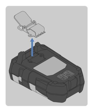
3. Remove the clip from the back housing.
