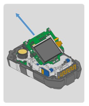
4. Lift the display PCBA and display assembly away from the main board at the angle shown. Discard according to local regulations.
