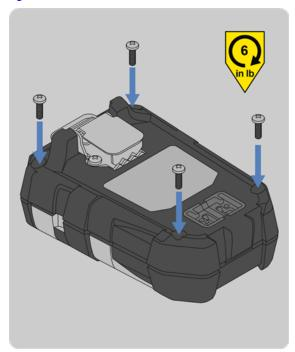
4. Install the four external screws with a Phillips head #1 torque screwdriver. Torque to 6 in-lbs (0.68 N-m).
