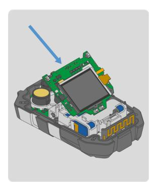
Take the display PCBA and display assembly, and insert the bottom left edge under the snap fit on the battery holder. Push the display PCBA down to engage the board to board connector.
