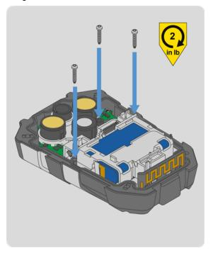
8. Install the three replacement internal screws with a Torx T6 torque screwdriver. Torque to 2 in-lbs (0.23 N-m).
