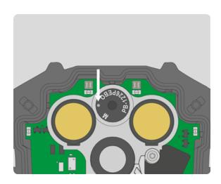
6. Install the replacement horn by pushing it down into the clear bracket.
