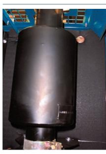
Integral, Ineris Certified Spark Arrested Exhaust Silencer. Up to MG 150SSP only
