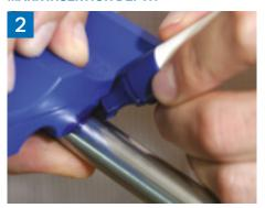
To ensure the pipe is fully inserted before pressing. Gives visual security.
