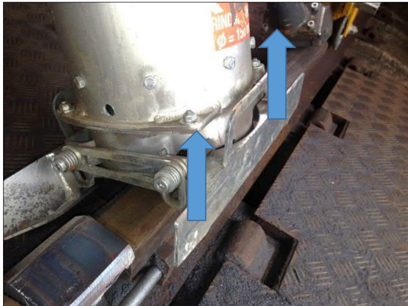
Fig. 85: Lift up spark protection (both sides)
