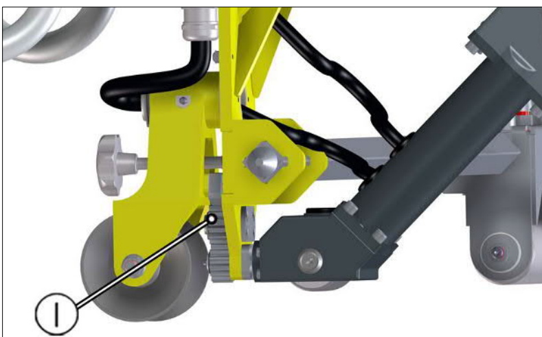
Fig. 95: Lubrication point gear wheels swivel mechanism (front side)
