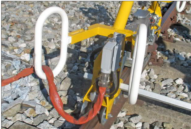
Fig. 48: Correct: Power supply cable threaded through one of the carrying handles
