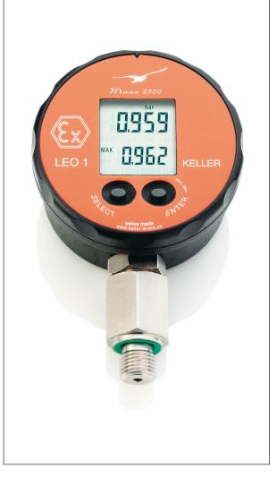
of measurement and neutralization of the stored extreme values at the start of an observation period. The easy-to-handle LEO 1 is available in an IP65 housing with four practice-based measurement ranges of -1...3 bar to 0...1000 bar. The optional protective cover allows outdoor operation in all weather conditions. This instrument is also available in an an Exia ATEX approved version compliant with 94/9/EC.
