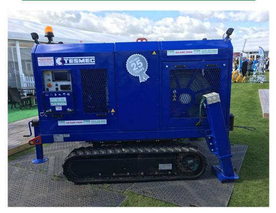
Our Winches are fully automatic, easy to use, reliable and simple to maintain. Built with the user in mind, they offer 'hands-free' operation. The operator simply sets the required tonnage and line speed and the Winch takes the strain. For swage lining and sensitive cable winching operations, an optional data logger can be fitted to the Winch to constantly monitor the line speed and winching force used. This then stores and prints a hard copy of the statistics for reference purposes.
