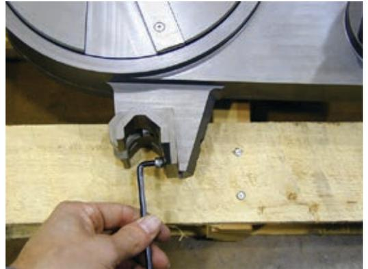
Attach rear guide rod bracket in the position shown.
