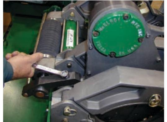
Lift facer out of the carriage and set on cardboard or wood blocks off of ground.
