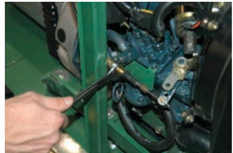
When the engine speed is adjusted, the hydraulic flow rate needs to be checked to verify it is within range.
