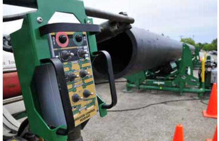
A remote control can be hung from the fusion machine, allowing a single operator to direct fusion and pipe loading operations.
