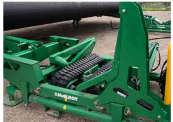
A tracked pipe stand nearest the fusion machine helps maneuver the pipe into the fusion machine.
