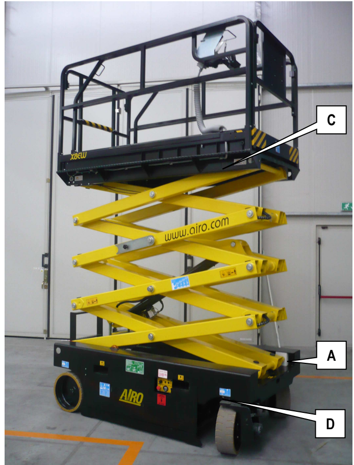
7-5: Location of main parts to be greased
