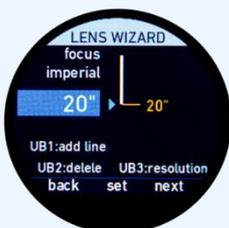
**FOCUS MAPPING** is not necessary for Cinefade operation but required to create a lens file and allows depth of field information to be displayed.
