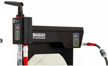
3. Daisy chain VariIND with cPRO camin and power source (see illustration below). It is also possible to use the cPRO motor as a RF receiver if no cPRO camin is available.
