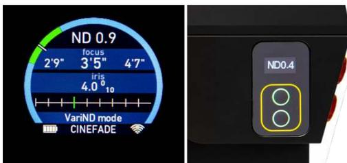
The current ND value is displayed on the hand unit display (use touchscreen to swipe between different information displays) and on the OLED screen of the Motorised Filter.
