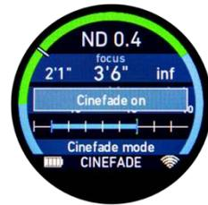
The VariND will automatically rotate back to ND0.4.
