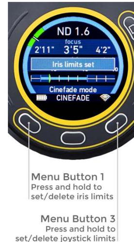
**MOTOR LIMIT VS CONTROL LIMIT** There are three different ways of limiting the travel of the iris slider and the rotation of the iris motor.
