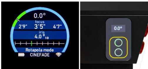
The current polarisation angle is displayed on the hand unit display (use touchscreen to swipe between different information displays) and on the OLED screen of the Motorised Polariser.
