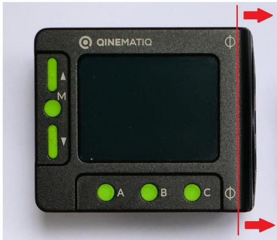
The reference mark for the distance „0m” is situated at the front of the BASE UNIT where the apertures for the ultrasound sensor are visible. The reference mark for the radio TAG is beside the qinematiq icon, also at the front of the device.
