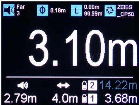
In case of a TAG distance value below 3m (= handover value – threshold) the merging distance value is calculated only from the ultrasonic distance.
