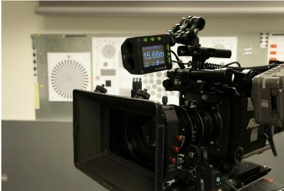
By default the SMART RANGER 2 display is situated at the right side of the camera but it is also possible to operate it on the left side of the camera.
