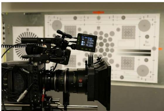
For fixing at the camera or at the matte box the SMART RANGER 2 BASE UNIT has 3x 1/4-20 UNC threads. With these the unit can be fixed to camera or matte box with common fixing tools.
