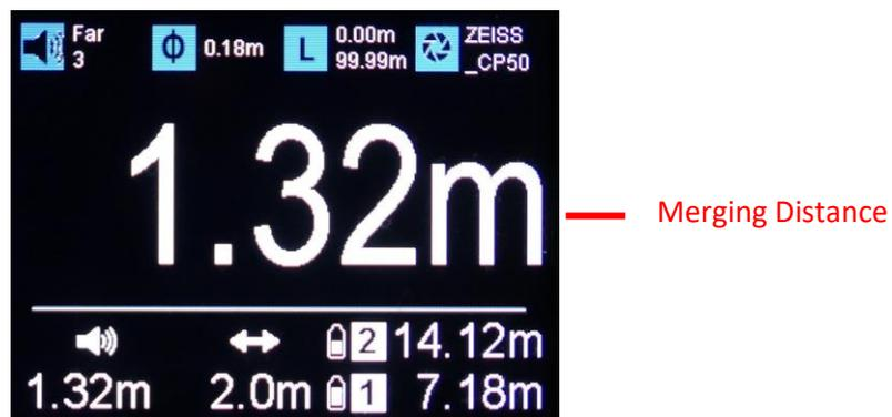
In close range the ultrasonic measurement is used as measurement value, in long range the TAG measurement. With SMART RANGER 2 it is possible switch between both measurement values automatically. Thus the merging distance values allow the permanent measurement of a motive that is moving from far range into close range.
