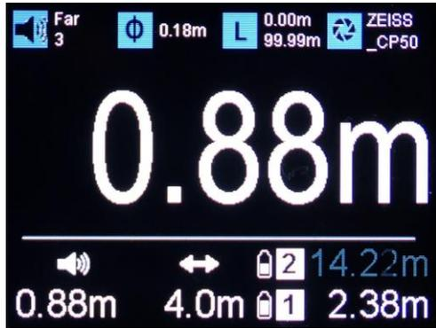
The single distance measurement readout shows the handover value between the ultrasound value and the distance value of the TAGs.
