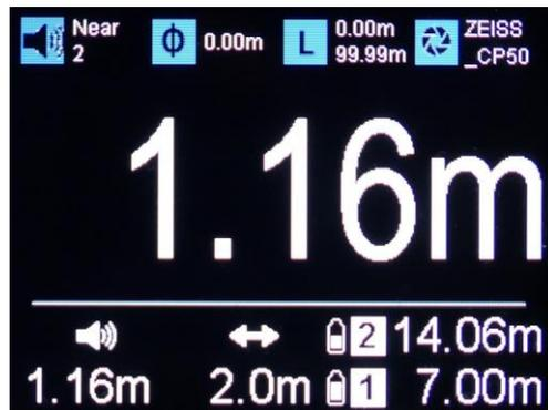
Also after switching on TAG2 the icon, the distance measurement value and the battery status symbol for TAG2 are visible.
