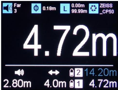
In case of a TAG distance value between 3m and 5m there is a linear transition from TAG distance to ultrasonic distance.
