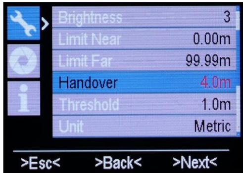
The handover value is adjusted by pressing the button SET B. When it starts to blink it can be changed by button UP/DOWN. Blinking stops automatically after 5s.
