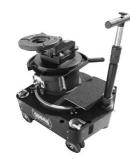
Steering column in low position without tracking bar.
