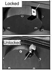
The center latch secures/releases the steering column.
