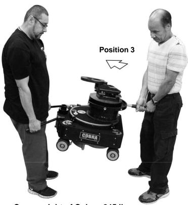
**Carry weight of Cobra: 245 lbs.** (Including weight of Leveling Head, Cobra Dolly and Lifting bars)
