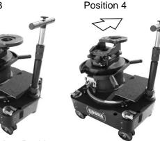
The 4-Way Leveling Swing Head has 48 locking positions. There are four (4) specially marked positions for easy recognition.
