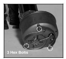
Using 5/8 in. Wrench, Attach tab to hex bolt.
