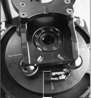
Note the engraved line on the 4-Way Leveling Swing Head. This should be lined up with the marker on the top plate to orient the head to the correct position.
