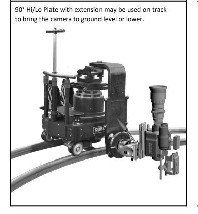
Adjust the column and engage the friction lock to set the camera at the desired height.
