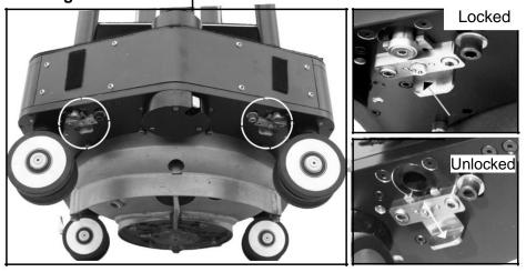
The left & right latches secure/release the tracking bar.
