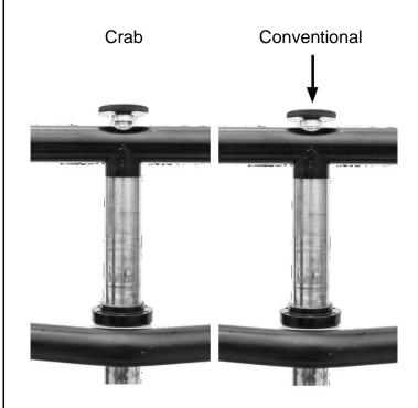
The default steering for the Cobra dolly is crab steering. With the wheels facing forward and the push-button engaged the Cobra will shift to conventional steering. When the push button is disengaged the Cobra will automatically maintain crab steering.
