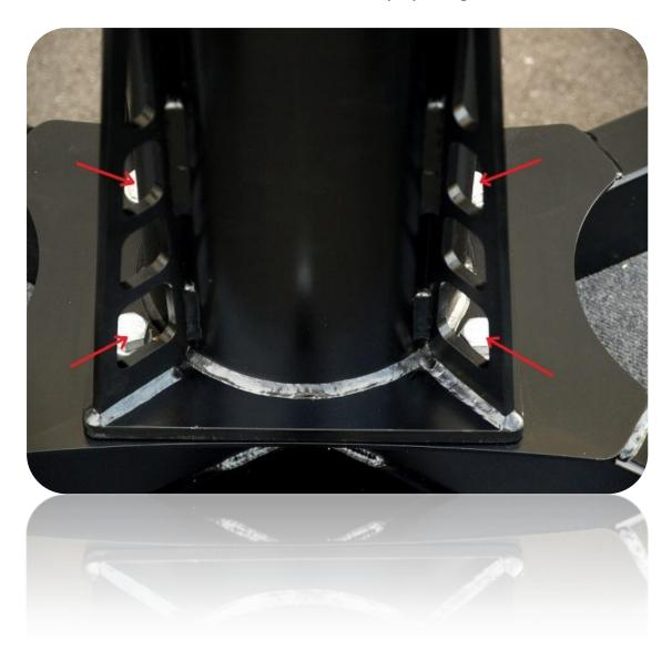
**C.2.** Also it's crucial to be sure that square receiver on the bottom of the column is properly engaged with the square shaft socket on the dolly.
