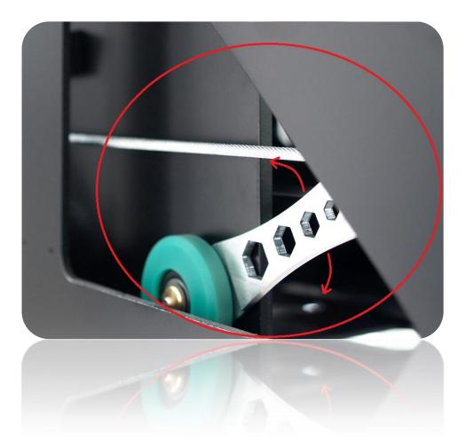
IMPORTANT: Electronics MUST be switched off before working inside of the arm. Also it is forbidden to move the sections during adjustment of crane mechanics. MovieBird does not take any responsibility if someone is maintaining the crane and don't abide above rules.
