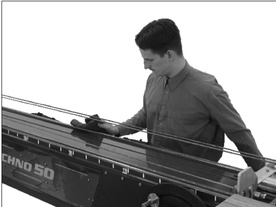
2.5.1.g - Cleaning the counterweight tracks
