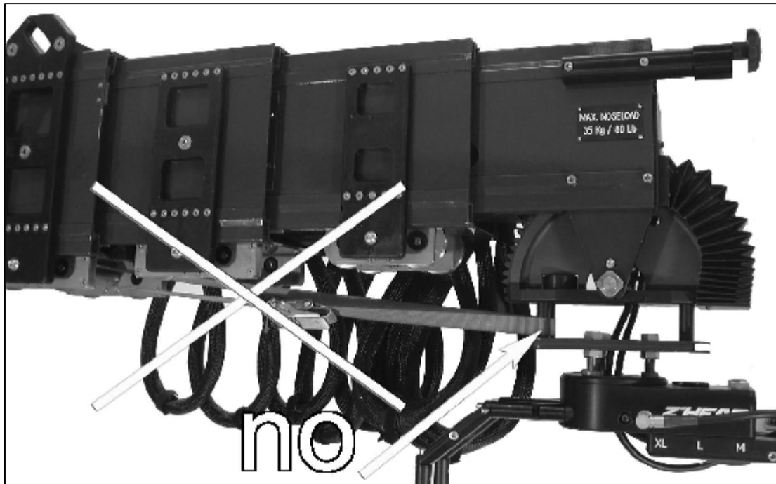
1.4.b - Strap at autohorizon – don't use like this
