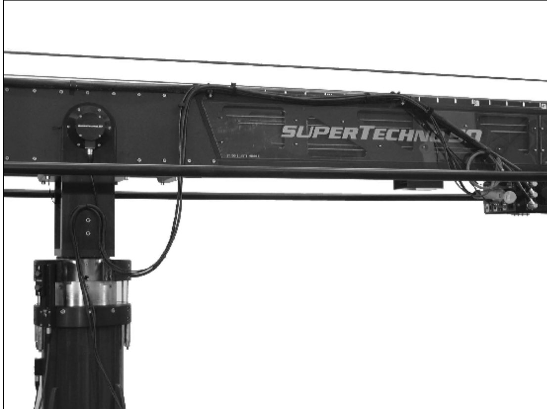
2.3.7. – Cable loop at fork
