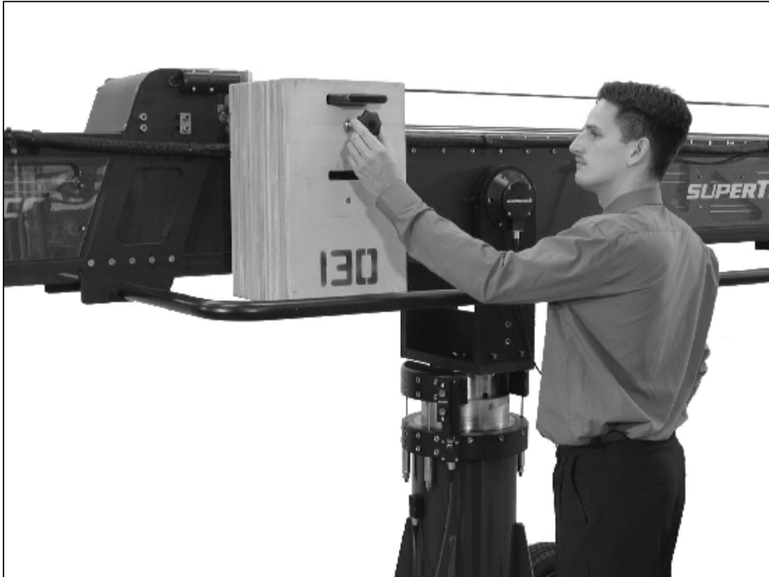
1.3. - Putting universal screw M 16x400 with nut at counterweights
