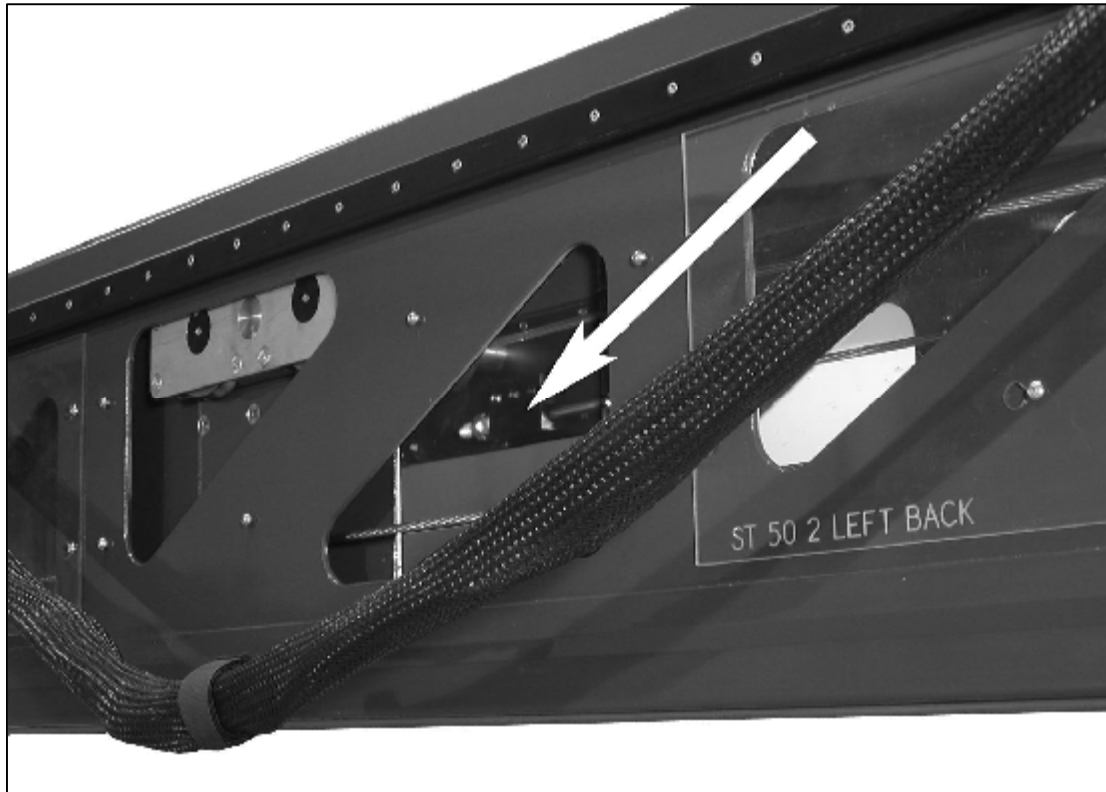
2.6.1.d - Anchorage pull in cable (3 rd beam section)
