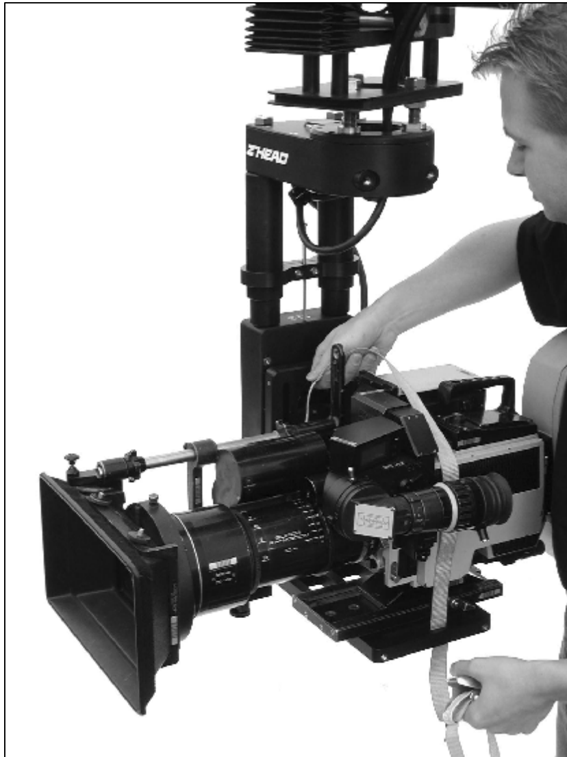
2.9.2.b - Securing the camera with a strap
