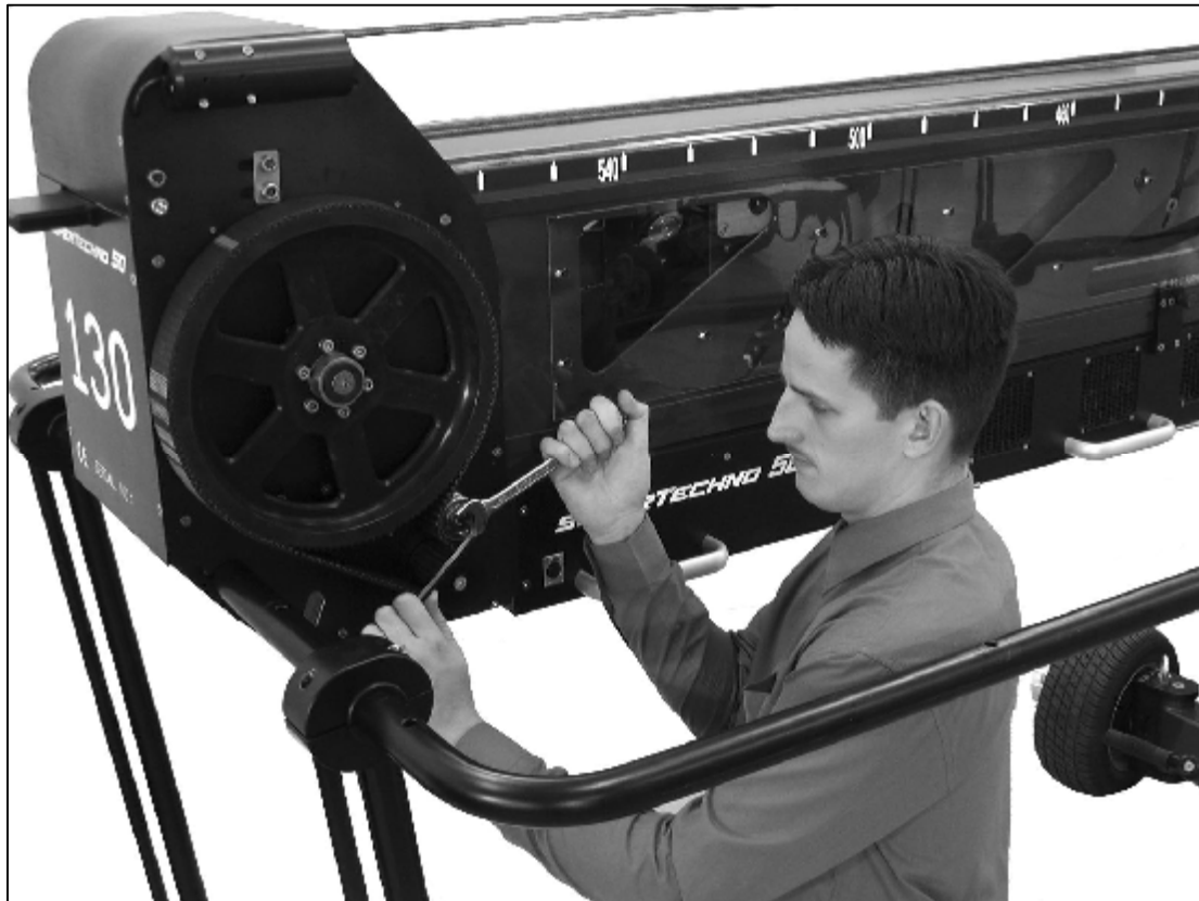
2.6.2 - Adjusting the eccentric pulley
