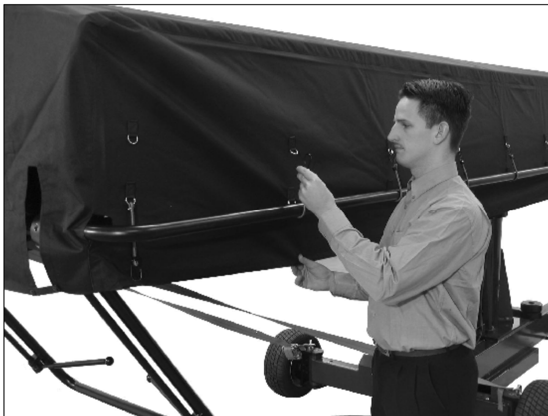
2.14.1.e - Fixing rubber band
