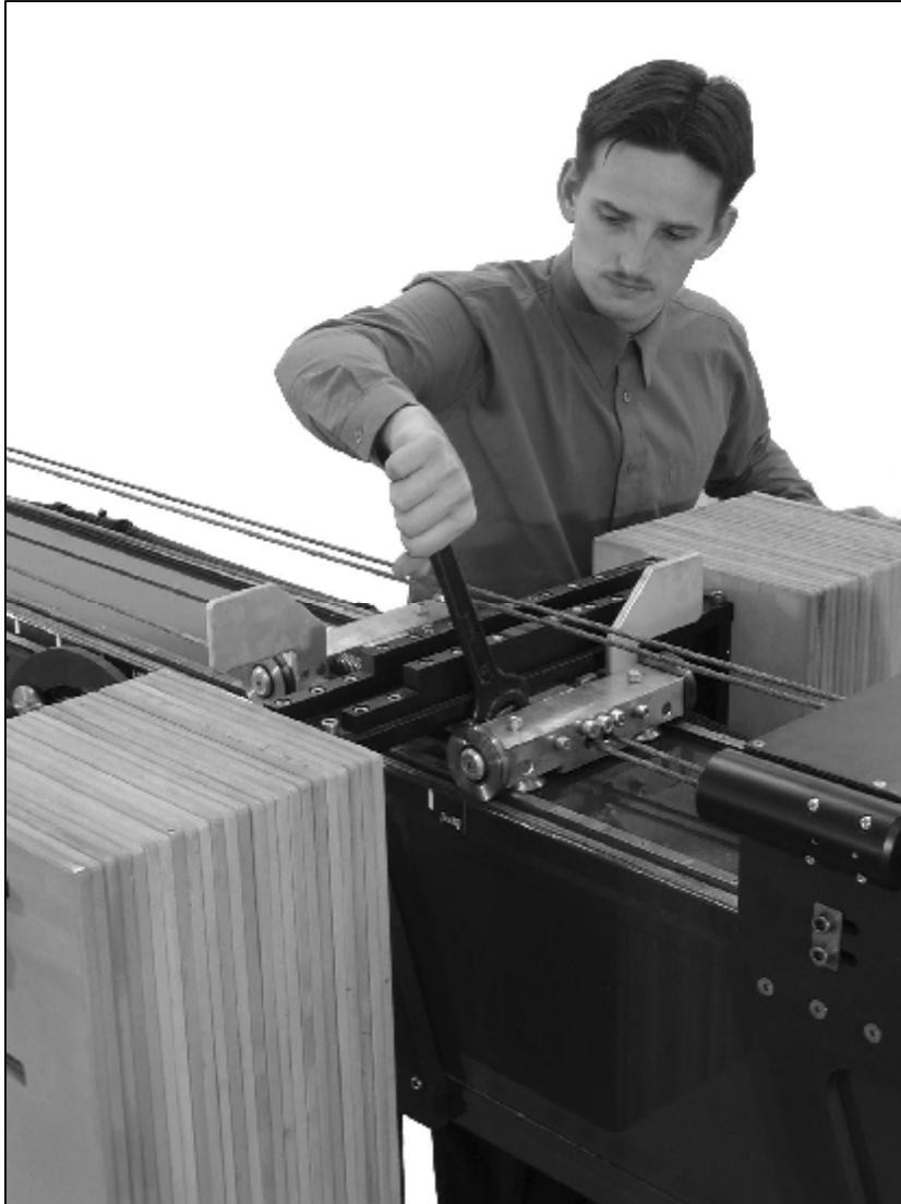
2.7.1.b - Adjusting the carriage
