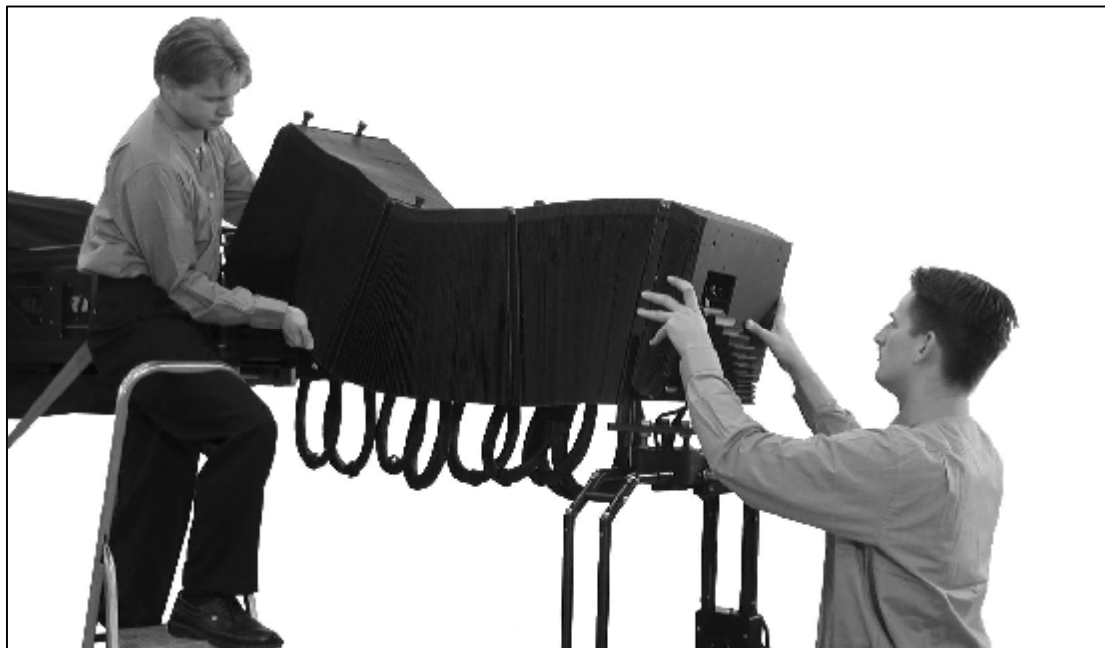
2.14.3.b - Putting bellows on the beams
