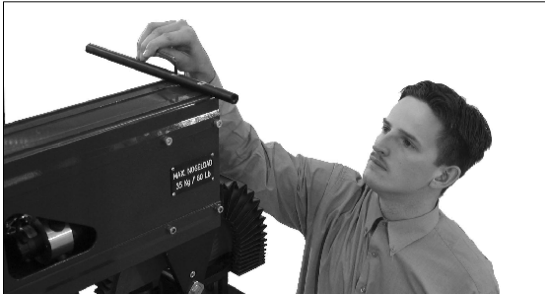
2.14.3.a - Fixing of shaft at fourth beam
