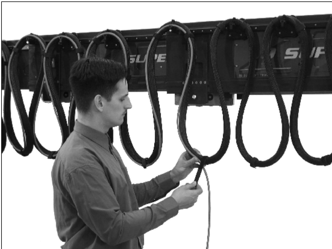
2.13.1.a - Mounting additional cables at wagon
