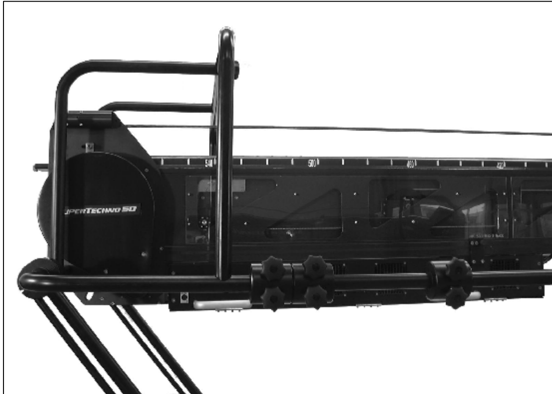
2.7.1.c - Sliding weights on crane
