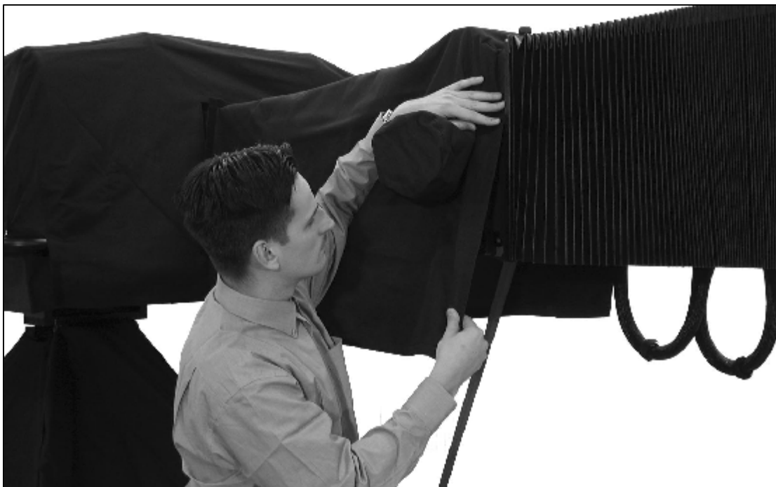
2.14.3.h - Fixing front part of cover for first beam
