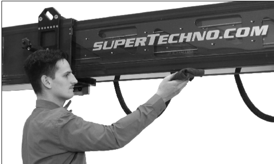
2.5.1.c - Cleaning tracks
