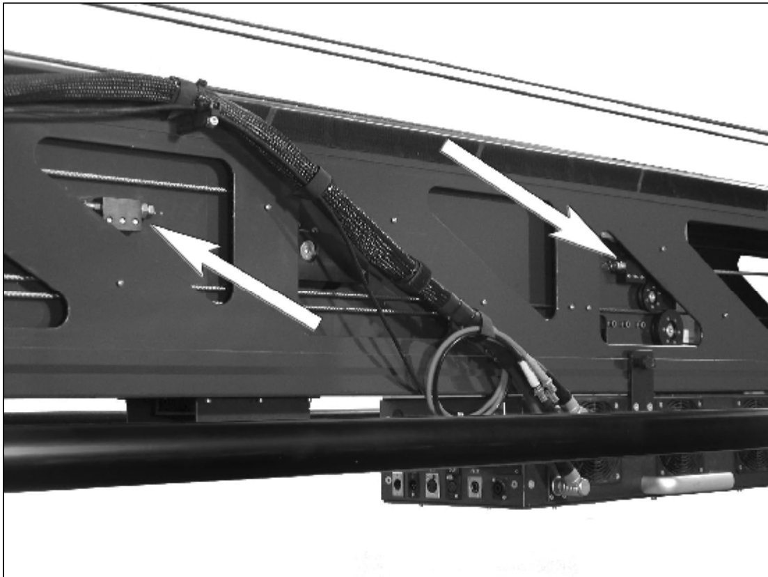
2.6.1.a - Anchorage pull in and out cable (2 nd beam section)
