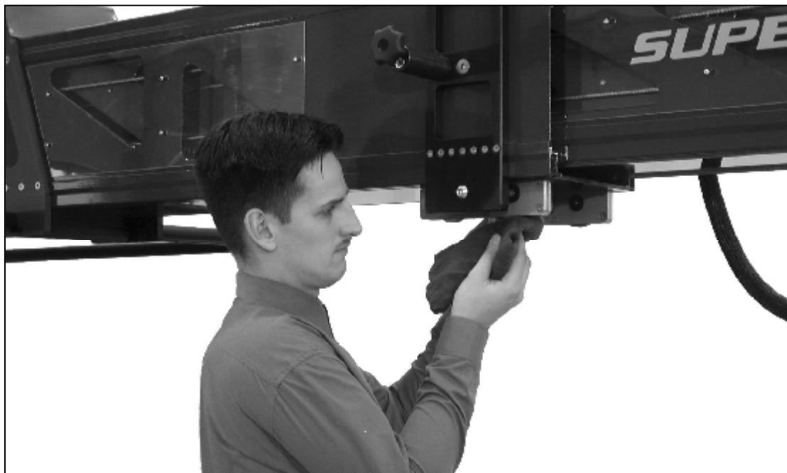
2.5.1.d - Cleaning rollers
