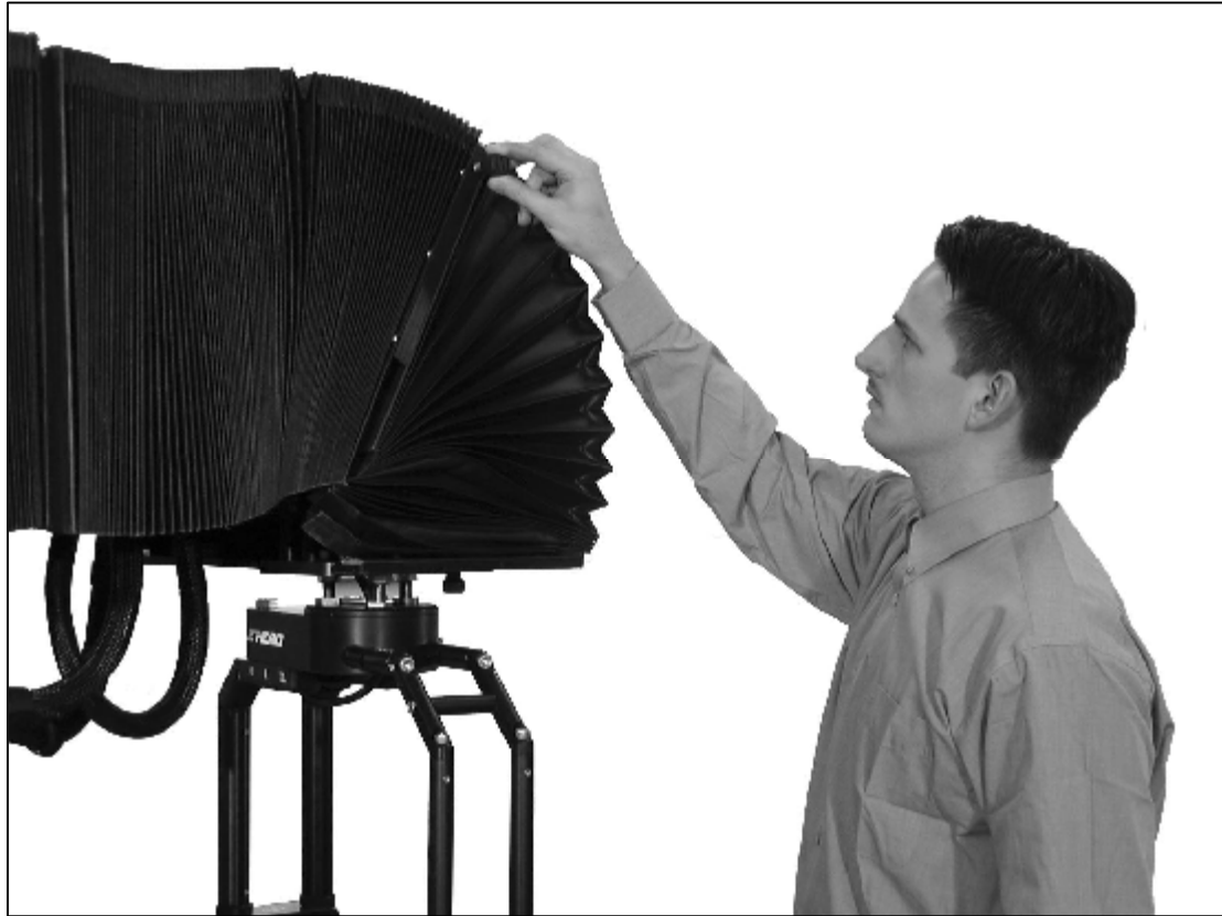
2.14.3.e - Attaching bellows frame at fourth beam
