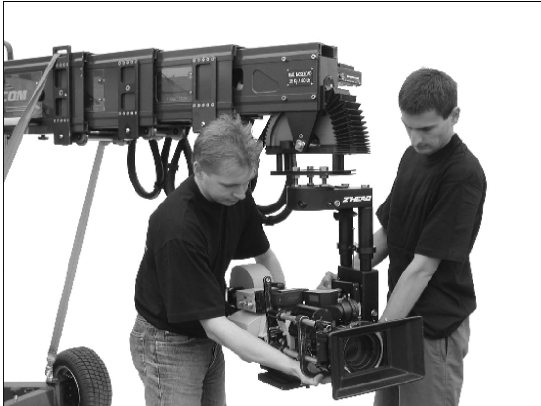
2.9.2.a - Mounting camera at base plate
