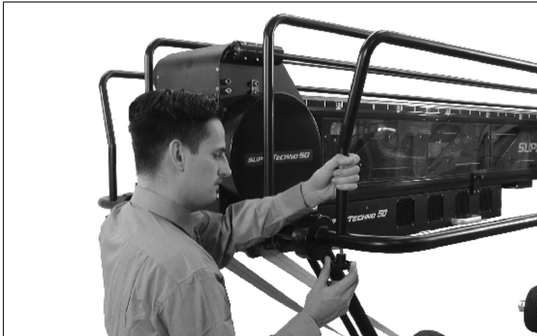
2.14.1.c - Screwing four tubes on railing
