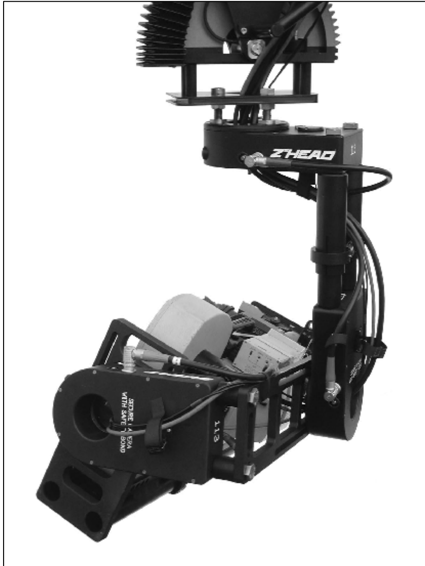
2.9.7.a - Cables at pan, tilt and roll
