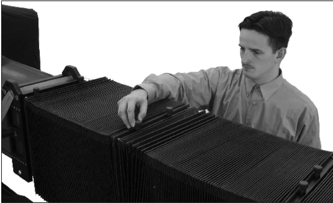
2.14.3.g - Mounting bellows frame on second beam
