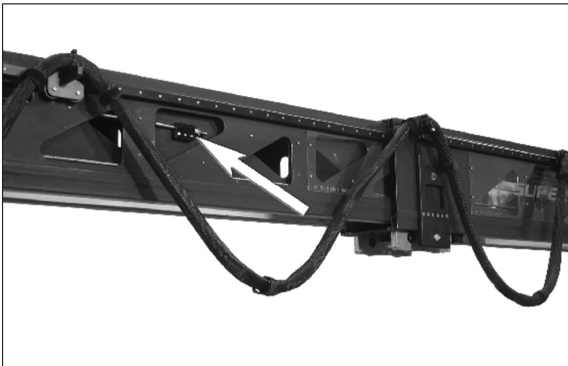
2.6.1.c - Anchorage pull out cable (4 th beam section)
