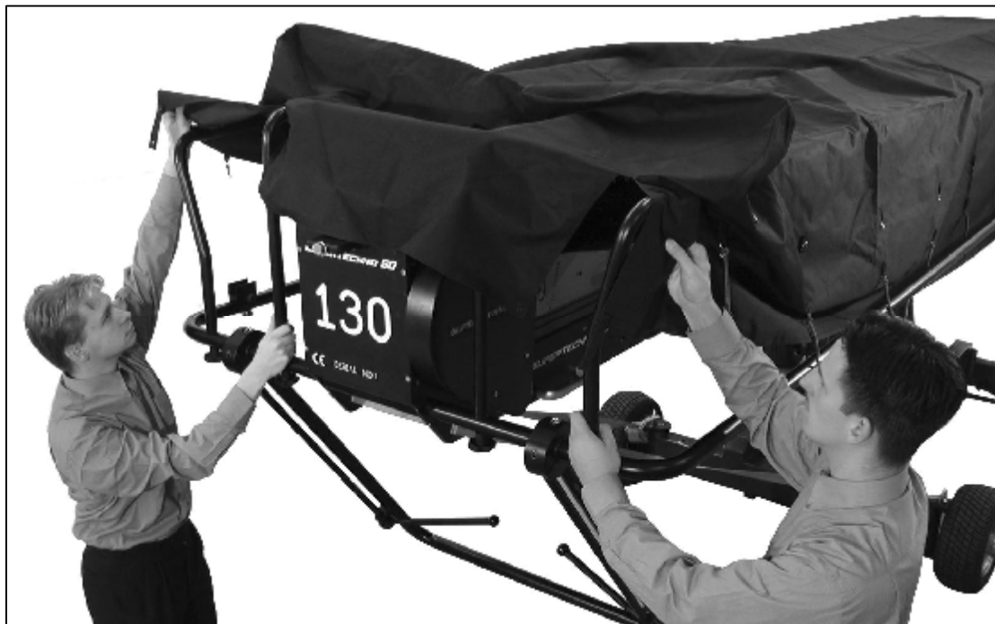
2.14.1.d - Putting cover over the first beam
