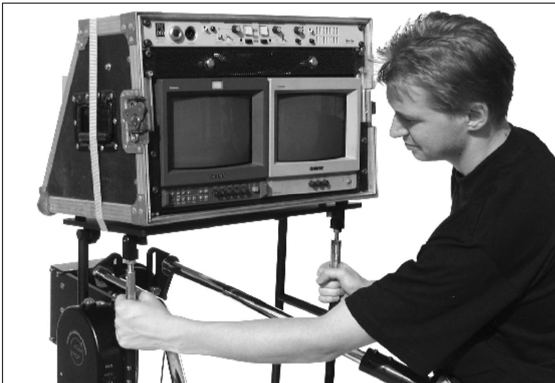
2.17.2.f - Setting the monitor angle with studs
