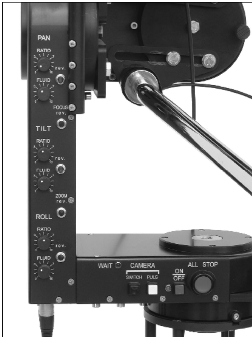
2.17.4.b - Front view of pan bars with potentiometers
