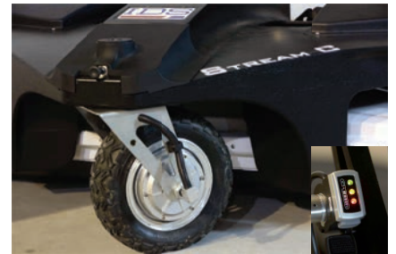
Stream C pivoting and motorized front wheel
