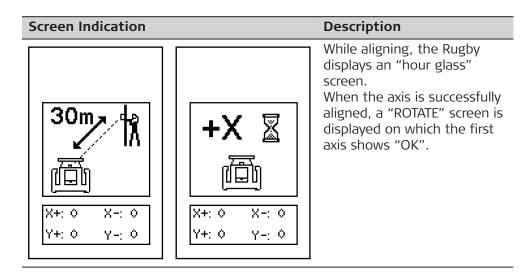
Step 2 - Rotate the Rugby 90° and align Y-axis (Y-) towards the Combo
