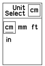
While a beam is being detected on the main screen, the digital read out displays the distance the beam is to the centre point on the Combo. Within the Unit settings menu, it is possible to select the units of the distance measurement:
