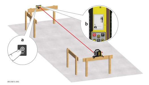
1. Use the Combo to move the rotating laser beam left or right until the Combo displays an on-grade position.
