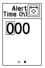
To be alerted of a calibration after X hours of use, enter the desired time before an alert appears.
