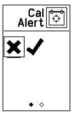
**Enable/Disable the calibration alert function** The calibration alert function is based on hours of use.
