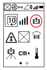
Press the Beam down option to check the alignment over a point.
