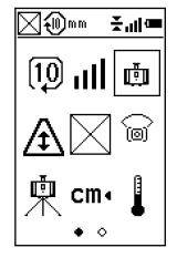
When the Rugby is moved to laydown position the beam down mode is activated automatically.
