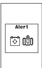
When the number of planned hours is reached, the calibration alert is displayed for 8 seconds. After calibrating the Rugby, the calibration alert hours are automatically reset. Changing or disabling the calibration alert is only possible by accessing the menu option "Calibration alert function".
