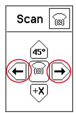
While in Scanning mode, the default direction of the scan is directly in the +X axis. Within the Scanning direction submenu, it is possible to control the direction of the scan manually.
