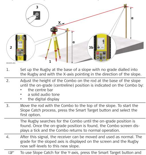
choose the second option. The process is identical.You can set up either one or both axes by using this procedure.
