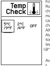
For each change in temperature of  $\pm$  5°C ( $\pm$  9°F) the Rugby returns to the level position to check if the change in temperature has led to a change of the main levelling system. For a more sensitive unit, you can change the setting to  $\pm$  2°C ( $\pm$  4°F) temperature change.
