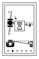
When the alignment procedure is successful, the Rugby displays the COMPLETE screen for 8 seconds, then resumes normal operation.
