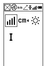
If there is no Rugby paired with the Combo a reduced menu screen is shown. This menu is limited to features that allow for the Combo to be used as a standalone receiver only.
