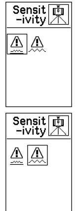
While levelling, the Rugby responds to disturbances, for example wind or vibrations, and stops the head rotation, if necessary. You can choose between two levels of sensitivity:
