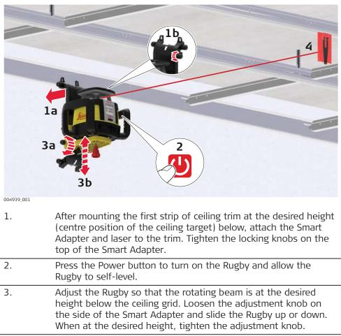
4. Install the ceiling grid using the ceiling grid target and laser beam as your reference.
