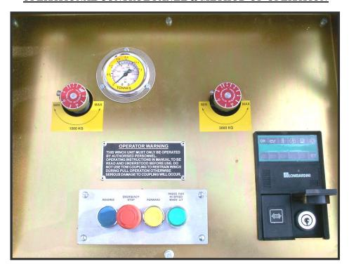
If the left-hand control only is used, the winch will only achieve a maximum line pull of up to 1000 Kg at high speed. If the pull exceeds 1000 Kg, the winch will stop automatically and hold load.
