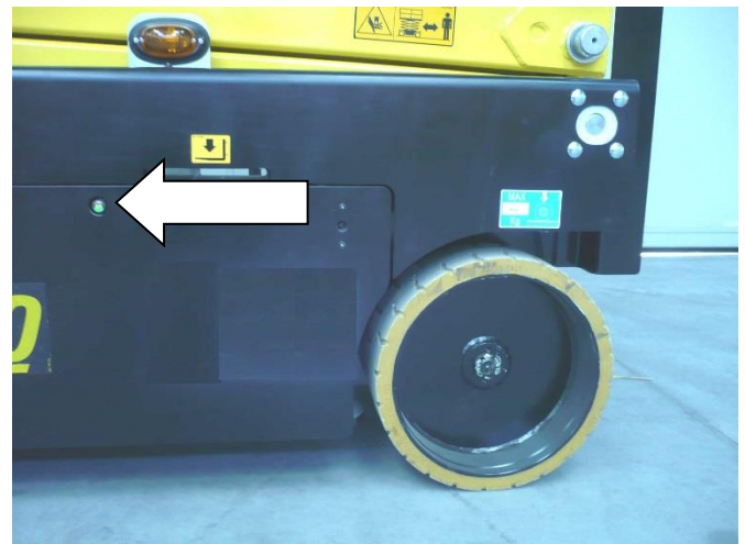
7-1510: Battery charger light
