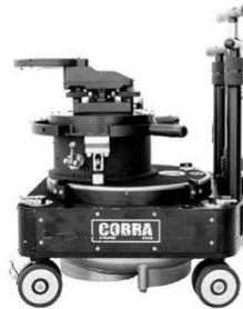
Steering column and tracking bar in low position.
