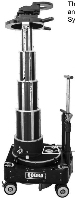
The Nitrogen Balance System is designed to balance the payload, providing a simple way of raising and lowering the telescoping column. Once the payload is balanced by the Nitrogen Balance System, the column and payload can be easily raised, lowered and stopped by hand.
