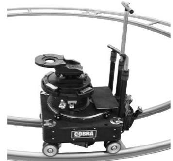
Steering column in high position and tracking bar in low position.
