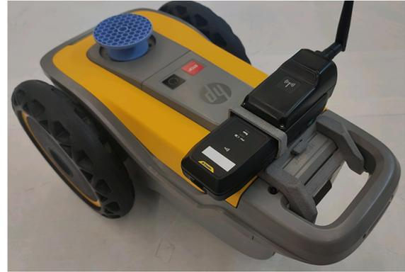
Ensure the antenna is facing down to avoid shadowing the prism.
