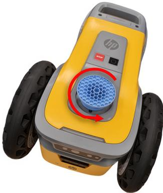
Turn the handle counterclockwise while pushing down.
