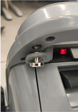
3. Insert the radio module into the holder and tighten the screw from below.
