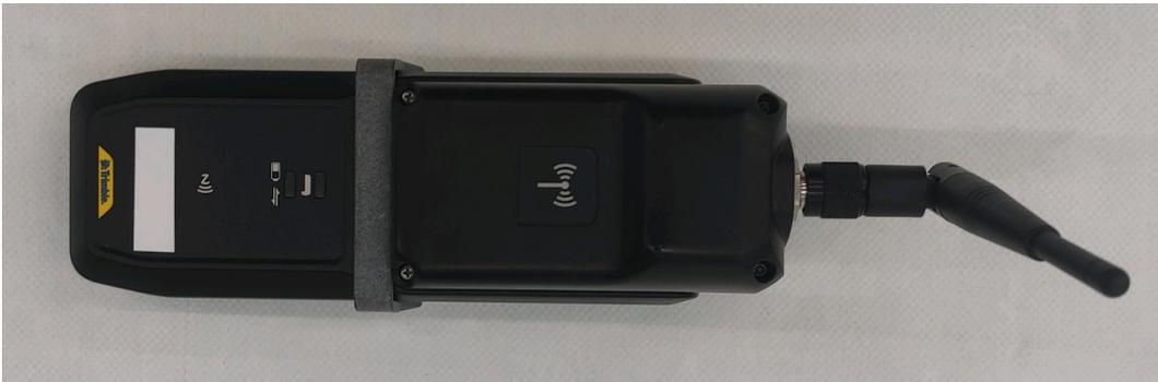
4. Slide the holder with the radio module into the rails of the locking system.
