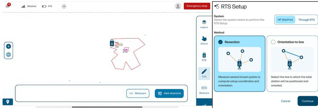
You can also choose between doing the RTS setup from the control panel or from the RTS screen when needed, or **Load a previous setup** if you have already set up your RTS.
