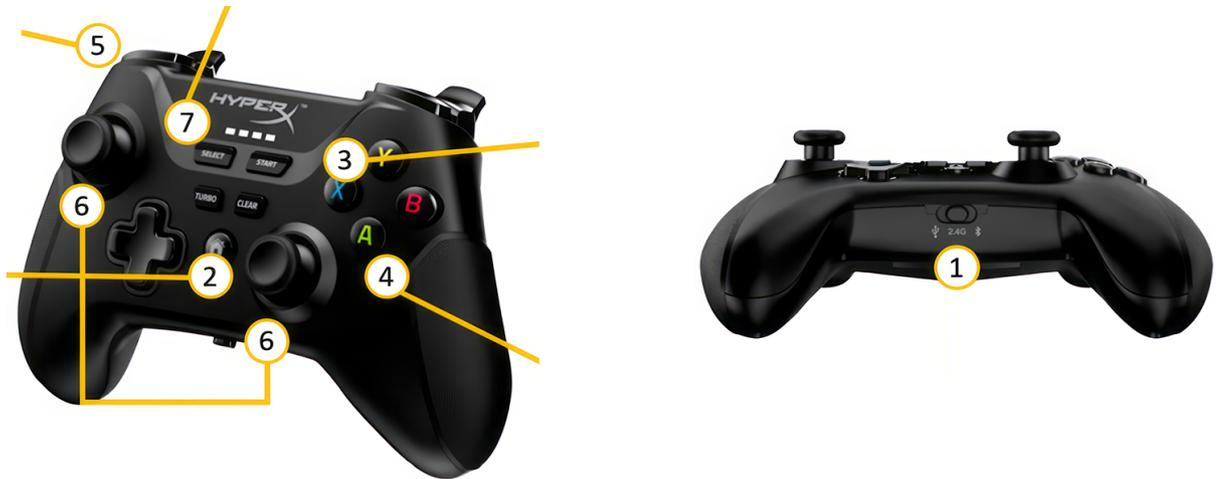
1. The switch must be set to Bluetooth position (right). To prevent battery drain, switch it back to USB position (left) to turn off the controller before storing it in the suitcase.
