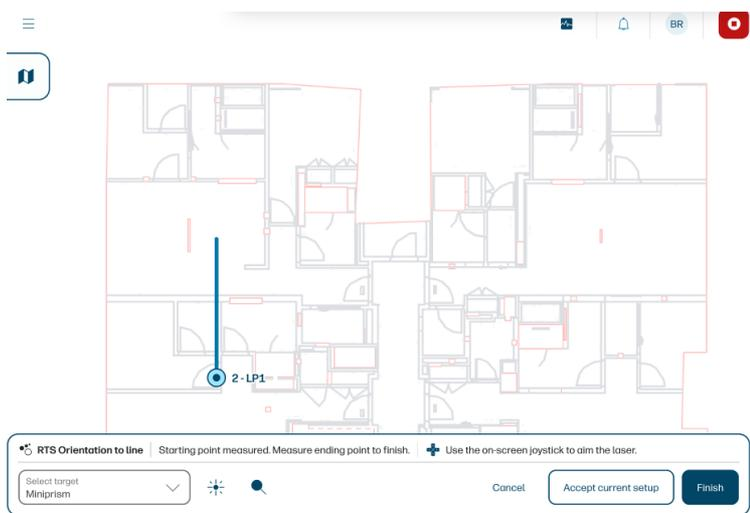
3. Tap the search icon 🔍 to ensure that the RTS has locked the prism, or ensure a good aim manually.
