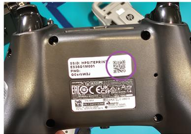
The Wi-Fi name is the same as the robot's serial number, which you can find on the label beside the printhead.
