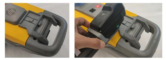
5. Press the button to allow it to slide fully in.
