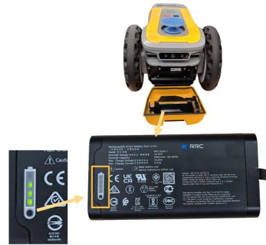
Press and release the button to check battery status.
