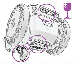
▲ CAUTION: Bear in mind that the fragile areas of the robot are the caster wheel, the printhead, and the front sensors. Handle the robot with care to protect them.
