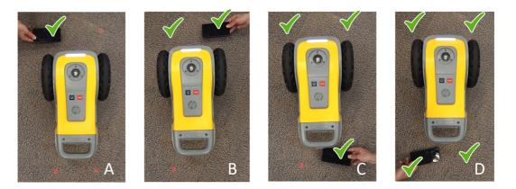
NOTE: This robot is equipped with a safety function to avoid falling over. Disabling this function may result in a hazardous operation. It is important to clean and maintain the sensors regularly as described in the maintenance instructions.
