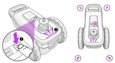
You should see four LEDs light up at the front and rear of the robot.
