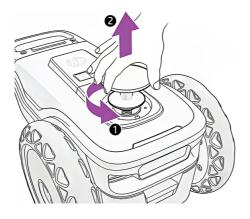
2. Insert the 360° prism and rotate it to secure it in place.
