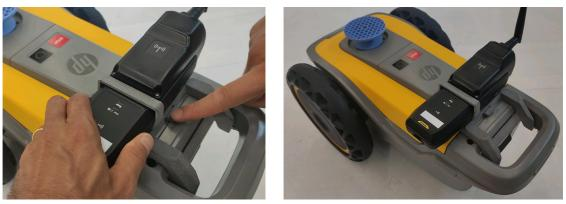
Ensure the antenna is facing down to avoid shadowing the prism.
