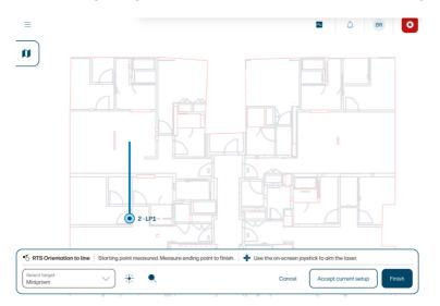
3. Tap the search icon • to ensure that the RTS has locked the prism, or ensure a good aim manually.
