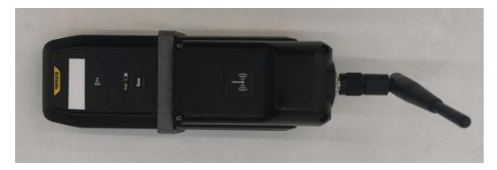
4. Slide the holder with the radio module into the rails of the locking system.
