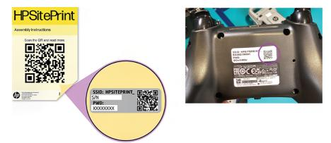
The Wi-Fi name is the same as the robot's serial number, which you can find on the label beside the printhead.
