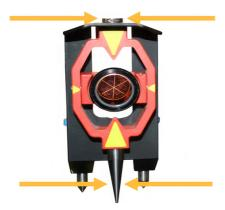
2. Set the bipod on the target points, and twist the blue leveling screws left or right to level it.
