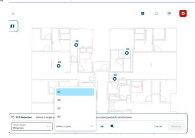
3. Before tapping **Measure**, tap the search icon **e** to make sure that the RTS has locked the prism, or ensure a good aim manually.
