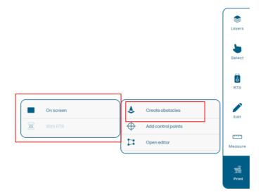
• With the RTS: You can add an obstacle by pointing the RTS directly at the physical location where you want to add it. You can choose between making a circle, a rectangle, or a polygon by selecting the correct prism.
