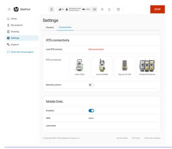
**IMPORTANT:** The prism selected in the user interface will override the model selected in the RTS. The user can restore the last RTS setup performed through the RTS tab in the Map view.
