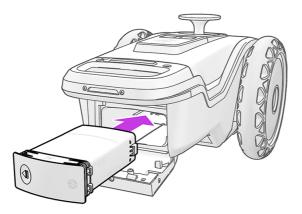
3. Press to the right to lock the cartridge in place.
