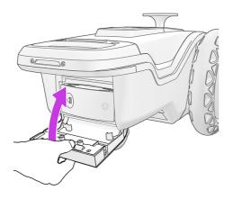
**IMPORTANT:** When replacing an ink cartridge for another one of different type or color, first insert a cleaning-fluid cartridge, even if the user interface does not request it.
