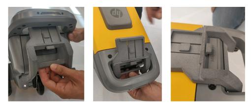
2. Attach the component underneath the handle with the two screws provided.
